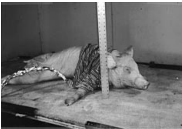
FIGURE 3 Typical carcass test. Metal scale (1.2m) supported by wire just above carpet. Thermocouple placed in neck area of carcass.
